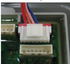
**Sensor Bars** - Disconnect harness and test Pink wire Pin 4 to Orange wire Pin 5. Approx  $\infty \Omega$  without laundry Approx  $190\Omega \pm 10\%$  with wet clothes
