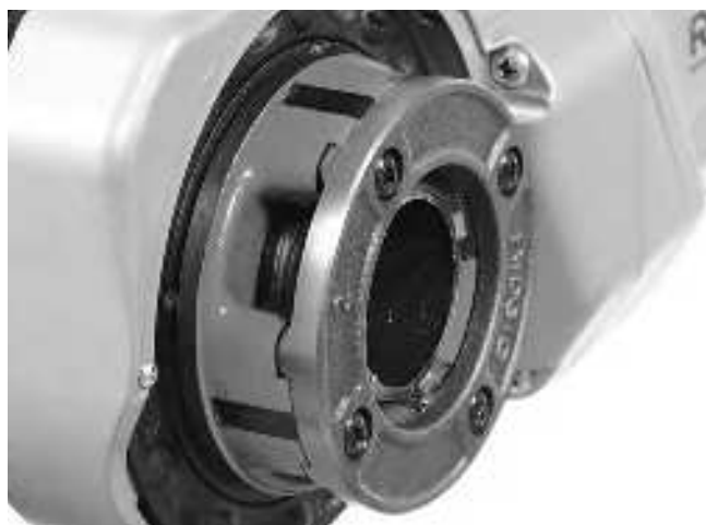
Figure 15 – Pipe Even with Edge of Dies
