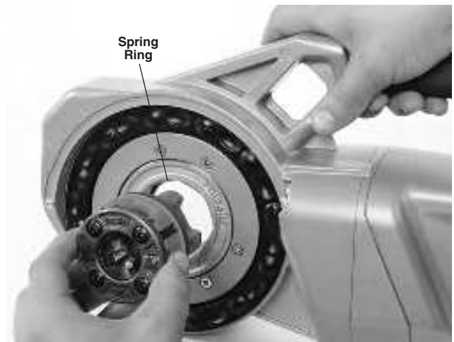
Figure 8 – Installing 1 1/4" or Smaller 11-R Die Heads (760 FXP 11-R only)
