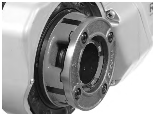
Figure 15 – Pipe Even with Edge of Dies
