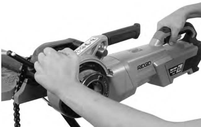
Figure 13B – Starting the Thread Using the Push Pad
