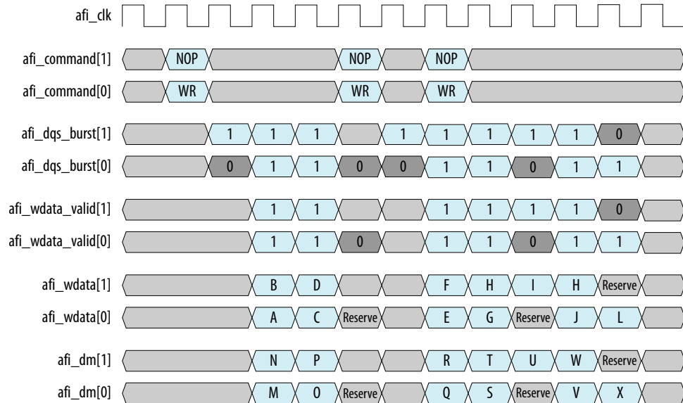
Figure 37. AFI Write Data with CRC Half-Rate, wlat=2
