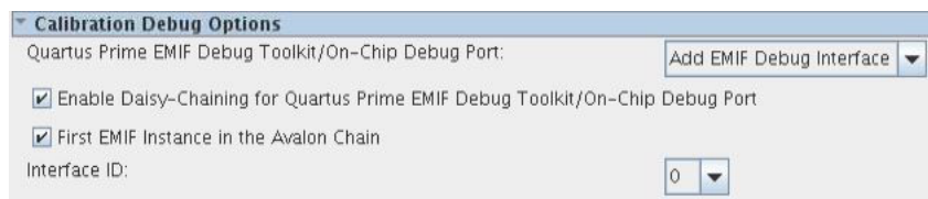
Figure 124. EMIF with EMIF Debug Interface and Daisy-Chaining Enabled
