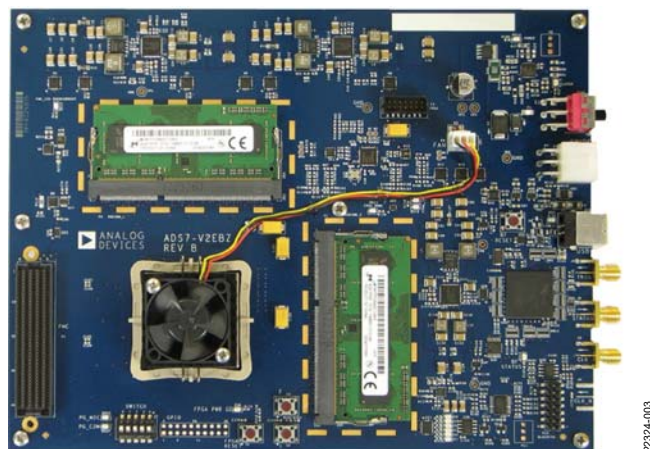
Figure 2. View of the Top of the ADS7-V2EBZ Pattern Generator Board
