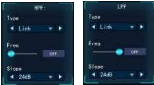
Main Function Setup: Channel High & Low Pass Filter Setup.
