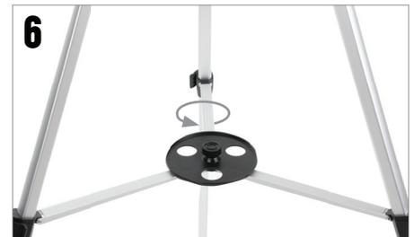
Place accessory tray on lower support bracket and then tighten fastener.
