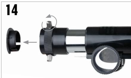
Loosen the set screws on the focuser and remove the plastic cap.
