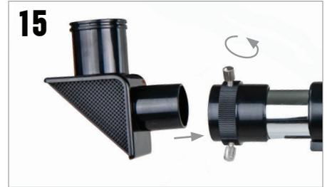
Insert the diagonal into the focuser and tighten the set screws to secure in place. Remove the plastic cap on the diagonal.
