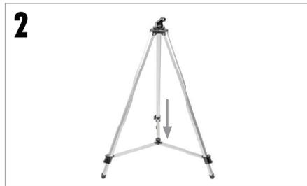
To set up the tripod, spread the legs outward until they are fully extended and push down center leg brace.
