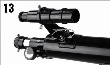
Replace the knurled nuts to secure in place and remove the lens covers.
