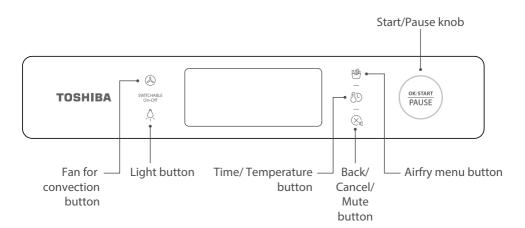
When the oven is electrified, the buzzer will ring once. The default function is AIRFRY. In the process of cooking, you can press "OK/START/PAUSE" to pause cooking.
