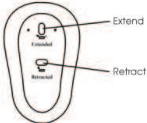
Note: if the remote controller is not working for the first time use, please press the Extended button on the handset to wake up the controller.
