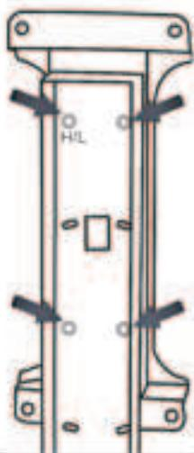
2. Place the support wallboard to be installed, mark the hole position and punch holes, put the expansion pipe into the hole, and fix the support body through the wallboard with the expansion screw.
