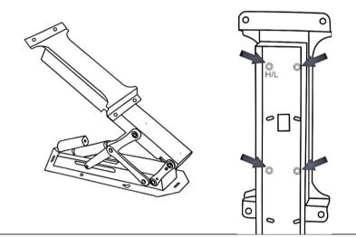
2. Place the support wallboard to be installed, mark the hole position and punch holes, put the expansion pipe into the hole, and fix the support body through the wallboard with the expansion screw.
