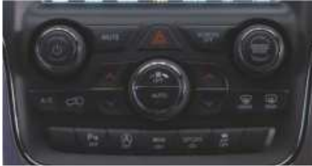
Automatic Climate Controls On The Faceplate
