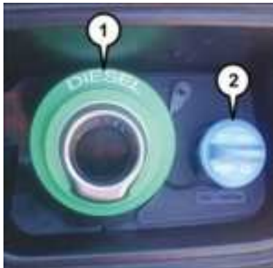
Fuel and Diesel Exhaust Fluid Fill Location
