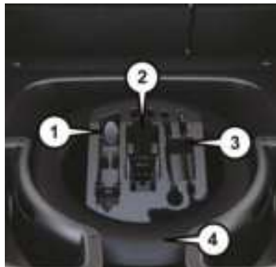
Fuel Fill Funnel/Spare Tire/Jack And Tools
