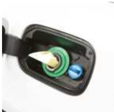
Emergency Fuel Fill Location
