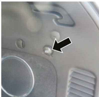
Rear Cargo Power Outlet
