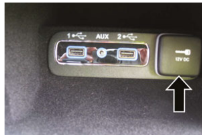
Front Power Outlet
