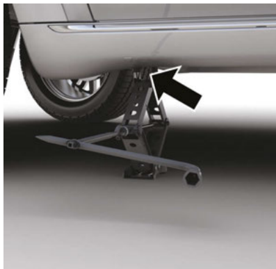
Front Jacking Location
