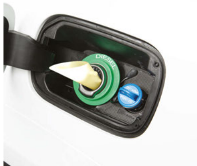
Emergency Fuel Fill Location
