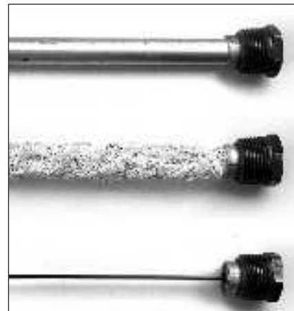
Figure 38 - Anode Rods from new (top) to partially depleted (middle) to fully depleted stages (bottom).
