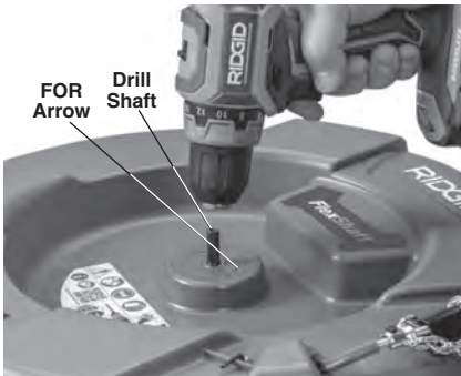
Figure 4 – Attaching Drill To Drill Shaft
