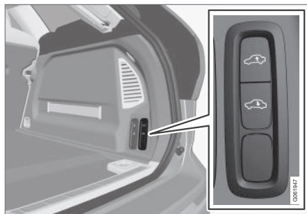
Controls for raising/lowering the car's rear section.
