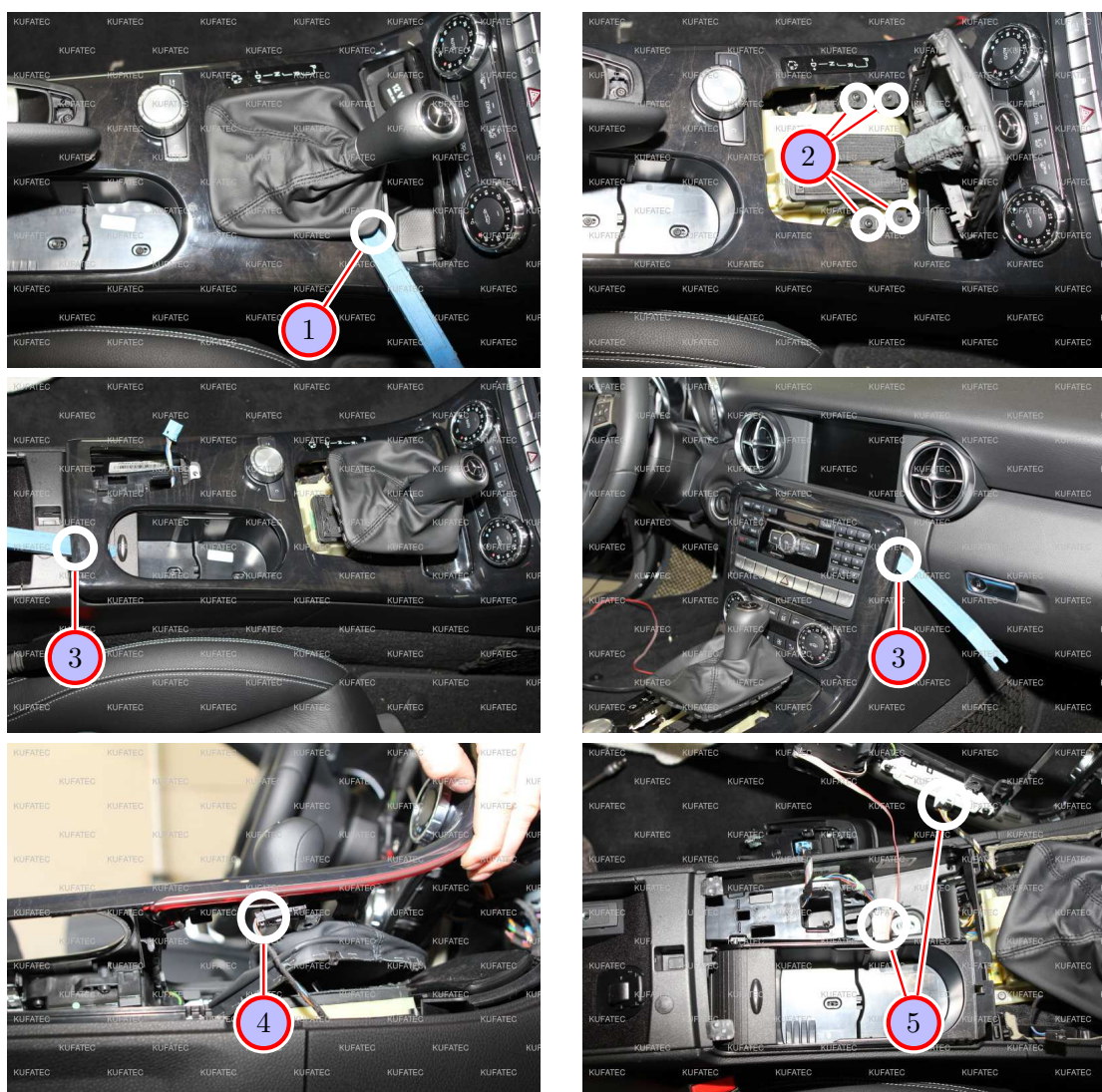
Figure 8: Removing center console
