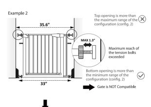
In this case, the supplied Up Cup (J) may be used to add the reach of the upper tension bolt. Please do note that for thick baseboards, the Up Cup may not be sufficient
