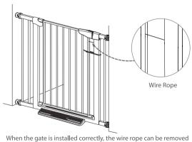
When the gate is installed correctly, the wire rope can be removed directly. When the wire rope cannot be removed, it means that it is necessary to tighten the tension bolt more.
