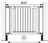
Top opening is more than the maximum range of the configuration (config. 2), so the user attempted to fit the dael attempted to fit the gate using config. 3 ABOVE the baseboard. This is dangerous.
