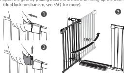
3. When the gate is opened between 30 to 90 degrees, the automatic door  $\,$ closer will close the gate. Successful closing is indicated by a click on the latch. The door will stay open when opened more than 90 degrees.
