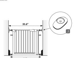
DO NOT attempt to fit the gate by installing above the baseboards. This will highly increase the risk of tripping and compromise the safety.
