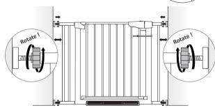
6.2 Make sure the left and right clearance between the gate and the wall is
