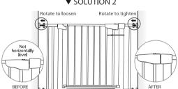
C. Gate is not properly aligned onto the door frame. Solution: Adjust the gate by loosening all tension bolts and repositioning the gate. Make sure the gate is properly aligned onto the door frame/door opening, then re-tighten tension bolts.
