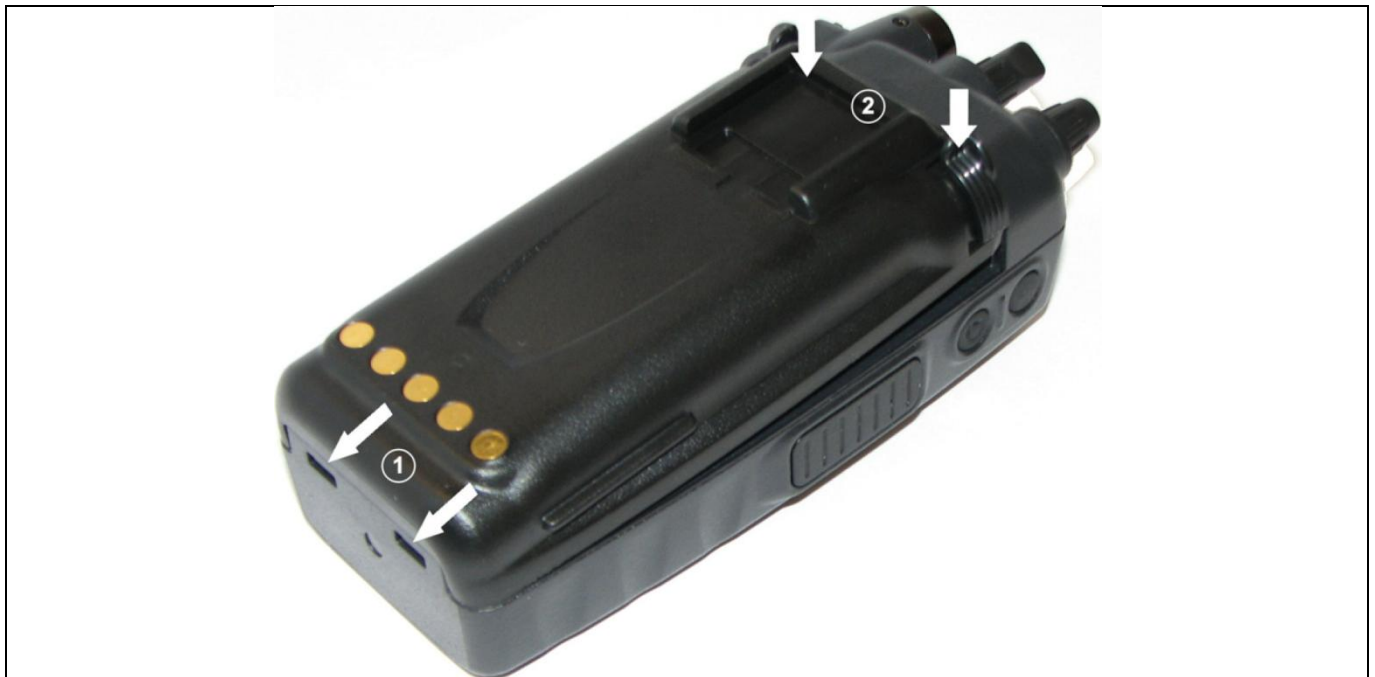
Figure 4-2: Attaching the Battery Pack
