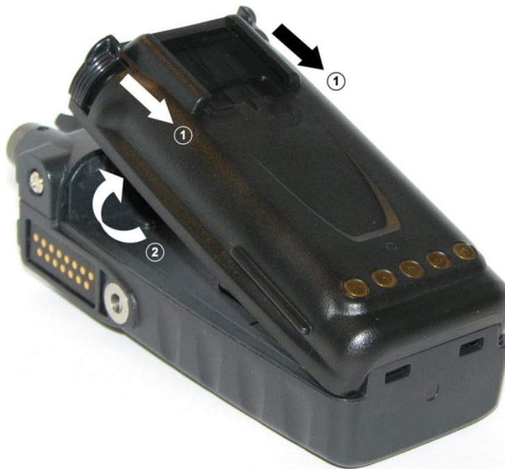
Figure 4-1: Removing the Battery Pack
