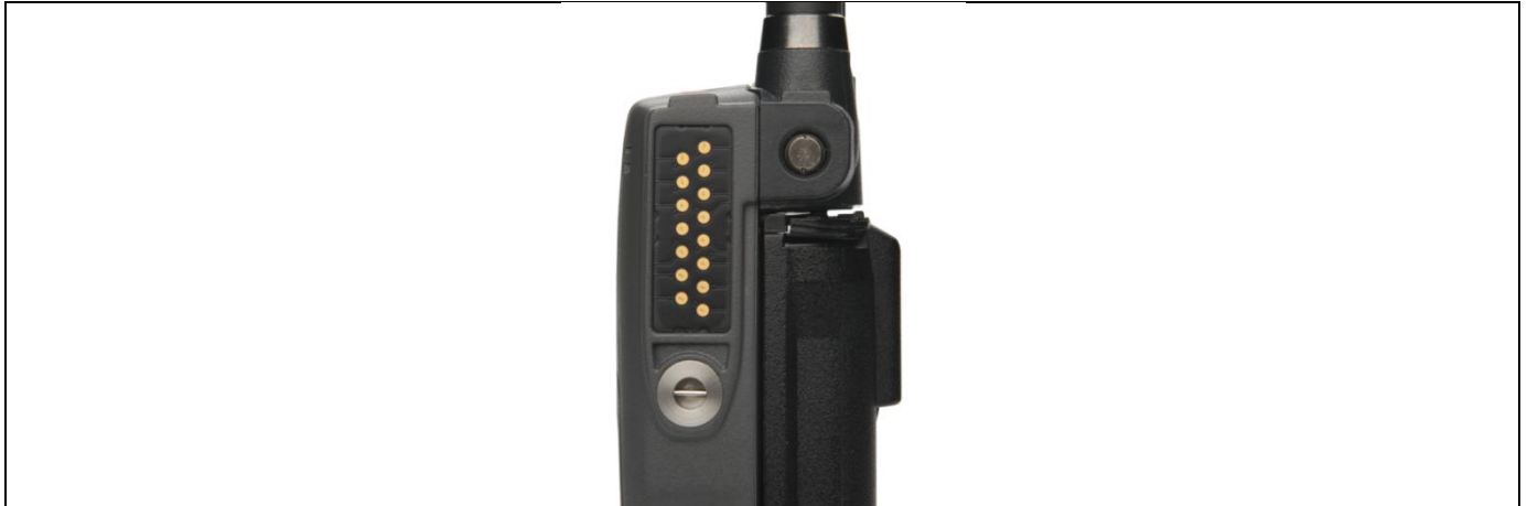
Figure 5-2: XG-15P 15-Pin Universal Device Connector
