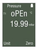
Displays Pressure reading in either millibars (mbar), kiloPascals (kPa), or inches of Water (inH2O)
