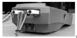
WARNING: - There is ONLY one correct way to connect the 'K' type thermocouple plug into the socket (see 2.4). The thermocouple plug is designed with one thick (negative) and one thinner (positive) prong. Forcing the plug into the socket the wrong way round may result in damage to the instrument. Failure to comply may result in damage to the instrument and will invalidate the warranty.
