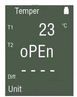
Displays Temperature reading of T1 in degrees Centigrade (°C) or degrees Fahrenheit (°F) Displays Temperature reading of T2 in degrees Centigrade (°C) or degrees Fahrenheit (°F) Displays the Differential Temperature (Diff.) between T1 and T2 in °C or °F
