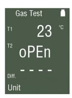
Displays Temperature reading of T1 in degrees Centigrade (°C)
