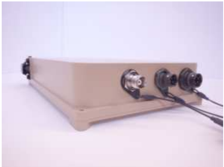
Figure 4-2 Installing Ethernet, Power and RF Cable
