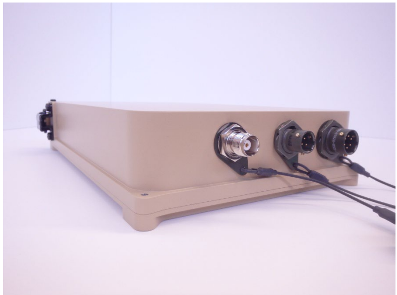
Figure 4-2 Installing Ethernet, Power and RF Cable
