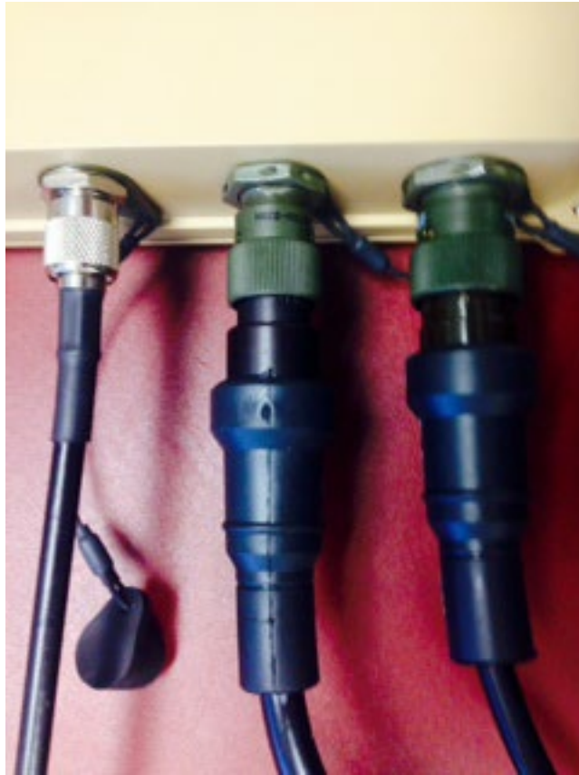
Figure 4-3 Cables Connected: RF, 3-pin and 6-pin respectively
