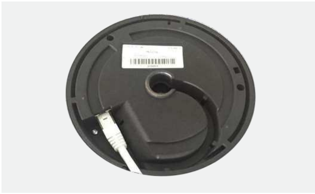
Figure 2: Beacon with CAT6 Cable on PoE Port
