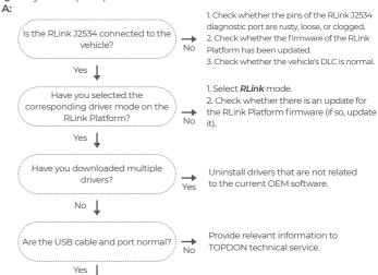
Check whether the USB port of the PC is normal, or try again with another port. Check whether the RLink J2534 hardware is normal.
