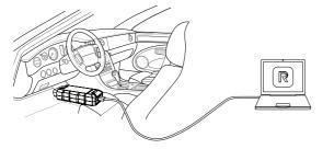
② Ensure that the communication is normal after the connection is completed. Then open the OEM diagnostic software and select *RLink* as the diagnostic interface.
