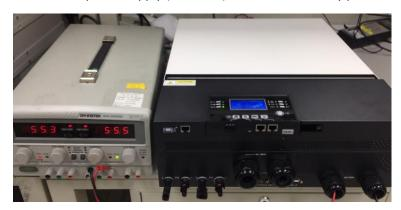
2. Turn on the Inverter which will working in battery mode.
