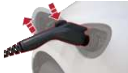
Removing The Charge Connector From The Vehicle Charge Inlet
