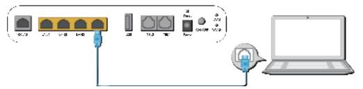
2. Set the IP address of the PC in the same subnet as the web address of the Huawei ONT. For example, if the web address of the Huawei ONT is 192.168.18.1 (for the web address of the Huawei ONT, see the product nameplate), set the IP address of the PC to 192.168.18.100.
