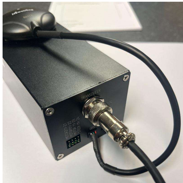
Where to plug the sonar into the back of the autopilot/fish finder receiver box
