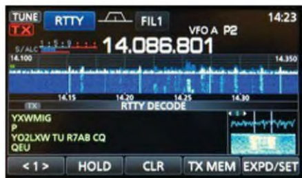
Figure 5 — The built-in RTTY decoder features a window on the lower right with a visual tuning aid — just line up the mark and space signals with the vertical bars. Up to four lines of decoded text are displayed at the lower left.
