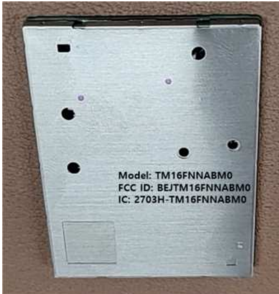
Installation of Shield-can cover
