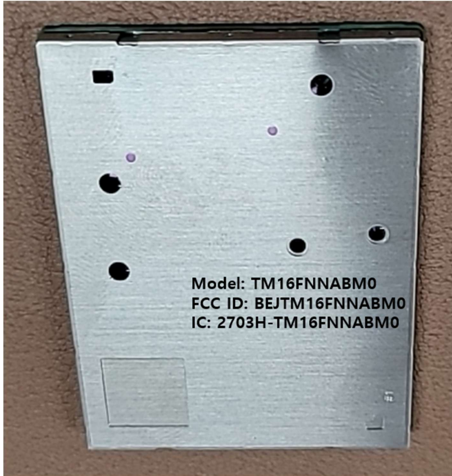
Installation of Shield-can cover
