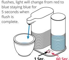
6. Once the flush is complete, light blinks blue for 5 seconds, then illuminate solid blue for 5 seconds.
