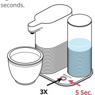
5. While red light is illuminated, press and hold dock button for 1 second. Light will blink red. While system flushes, light will change from red to blue staying blue for
