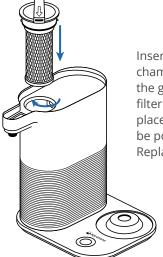
Insert the filter with the attached filter. chamber cap onto the chamber so that the grooves of the cap line up. Twist the filter chamber cap to the right to lock into place. Arrow on filter chamber cap should be pointing towards the dispenser end. Replace the filter housing lid.
