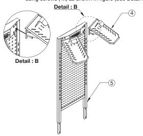
Step 4: Attach thr Top frame (5) to the Bottom frame (3) by using Screws (4x) as shown in figure (See Detail : C).
