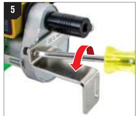
Remove the existing bracket screws and nuts from the motor drive housing. Be careful not to lose the small parts—set the screws and nuts aside in a container for safekeeping.
