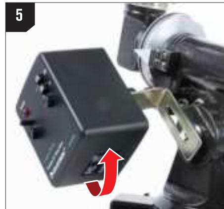
Align the slotted hole on the motor bracket with the threaded hole where the Allen screw was. If necessary, pivot the RA worm shaft by rotating the connected motor drive. This will rotate the shaft until the slotted hole in the bracket aligns with the threaded hole on the mount.
