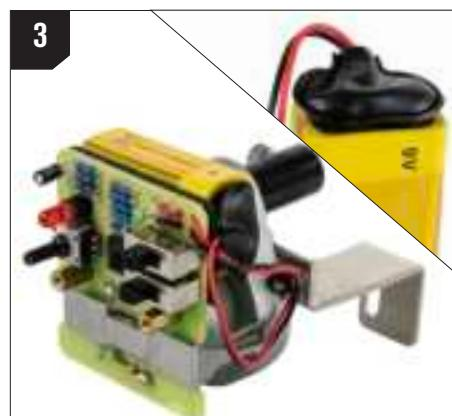
Connect the battery to the wire harness inside.
