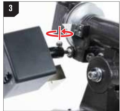
Tighten the coupler screw onto the flat side of the shaft using a flathead screwdriver (not included).
