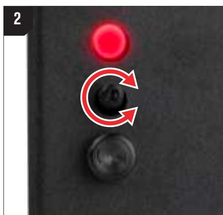
Turn the speed rate regulator (H.) clockwise to increase speed or counter-clockwise to decrease speed.
