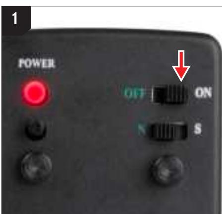
Slide the On/Off switch (I.) to the "On" position. A red LED will illuminate.
