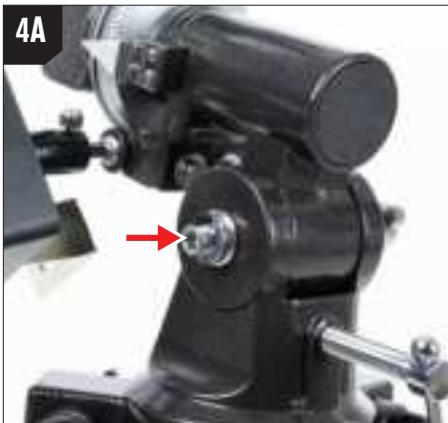
Locate the 3/8" Allen screw on the polar shaft and remove it with the included 3/8" Allen wrench. On the CG-2, it's opposite the latitude scale.
