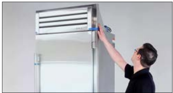
FIG. 2. Inspect the unit's exterior for visible damage.
