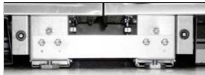
FIG. 18. Installed joining bracket.
