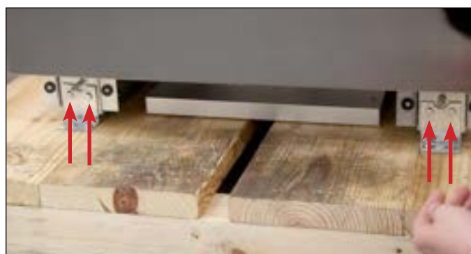
FIG. 7. Shipping bracket bolt locations.
