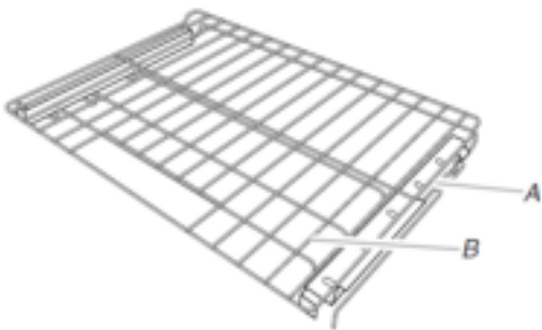
A. Rack frame B. Sliding rack
