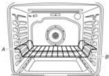
A. Ends of rack in position 3 B. Food in position 2
