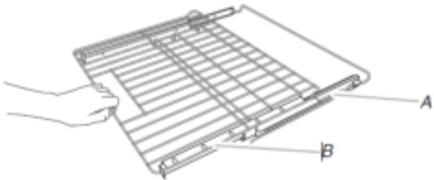
A. Rack frame B. Sliding rack
