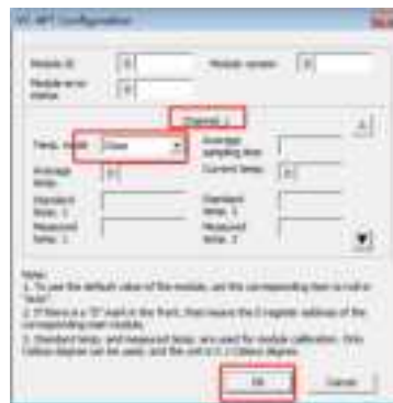
Figure 4-1 First channel setup
