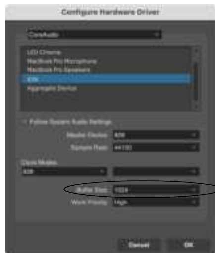
Figure 7-2: In Digital Performer and Performer Lite, choose Setup menu> Configure Audio System> Configure Hardware Driver to open the dialog shown above and access the Buffer Size setting.
