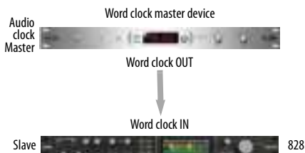
Figure 4-12: Slaving the 828 to word clock. For the 828 clock source, choose Word Clock In .
