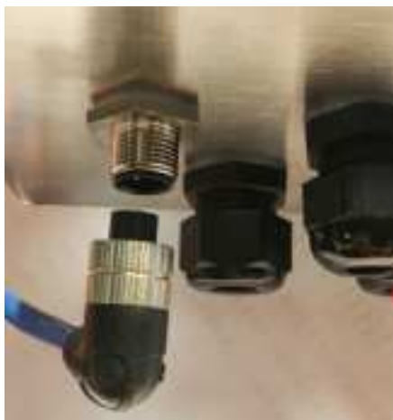
Figure 3. Cable Connection to the 882IS
