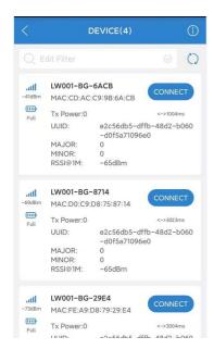
After the device is turned on, the device Bluetooth will start broadcasting. Open the MKLORa APP and choose LW001-BG PRO, then you can search the LW001-BG PRO device by click the refresh icon. The default broadcast name of the device: LW001-BG PRO-XXXX.
