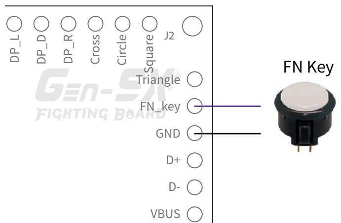
\*To use Turbo, RGB LED adjustment, and other settings with hotkey operations, it is necessary to connect an external FN key.
