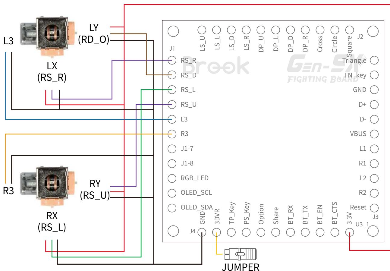
\*If a digital-analog joystick is installed, the stick will not be able to switch between RS/LS modes.
