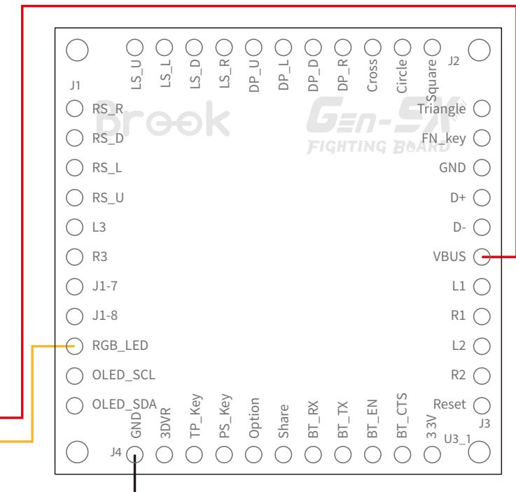
\*The order in which the RGB lights on the buttons illuminate will follow the wiring sequence. For example, the first connection will be numbered as 1, and so on.
