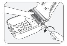
2. Remove the gear and impeller, clean any debris, and then reinstall them.
