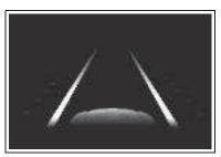
Indicates that the system is recognizing white (yellow) lines or a course\*. When the vehicle departs from its lane, the white line displayed on the side the
