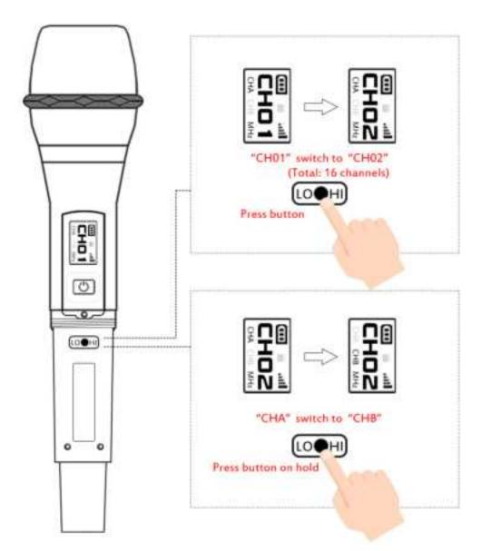
2. Press the HI-LO button ④, the frequency on the screen will be changed.
