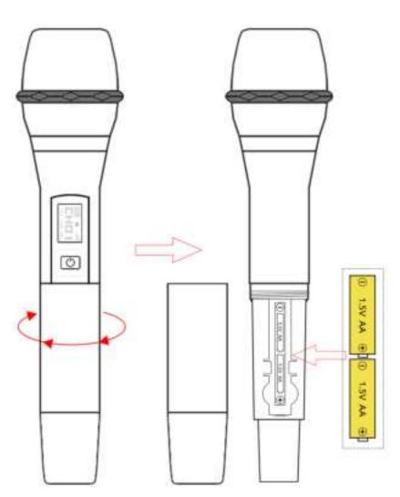
Install 2\*AA batteries before using the wireless microphone and installing instruction is as follows:
