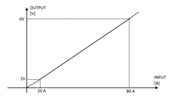
Note that with an input of 0 A the output is 0 V and over 80 A the output is over 6V (6V and 2V are not a limit).
