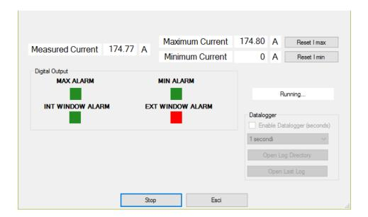
The test configuration will acquire the measure from the Modbus registers, you can also reset the MIN/MAX values.
