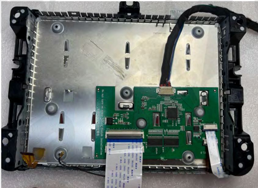
14. Run the provided 'LCD-OUT' cable through the hole in the chassis from step 13 and connect to the PCB NOTE: pins face UPWARDS)
