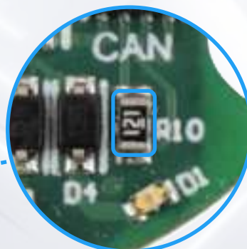
The resistance of the bus terminal is 120Ω
