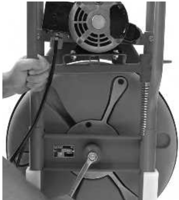
Figure 18 – Removing Drum Bolt
