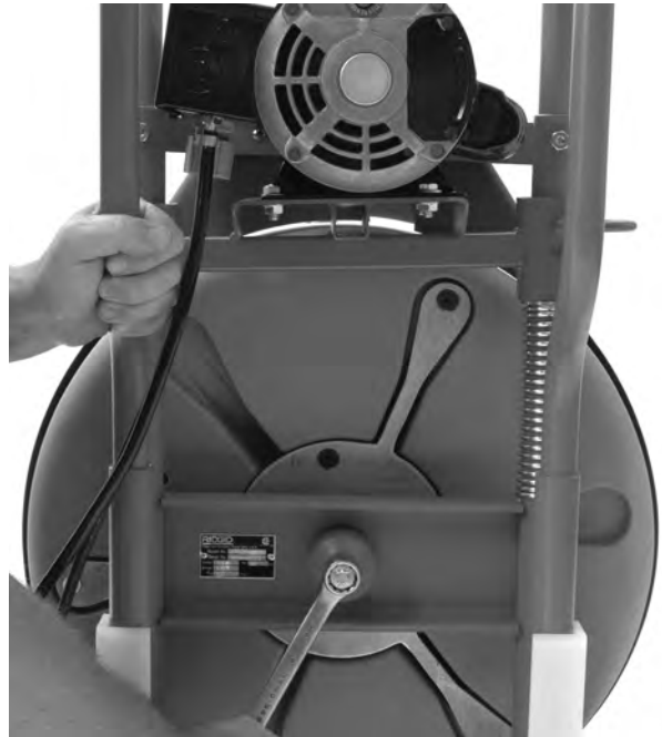
Figure 18 – Removing Drum Bolt
