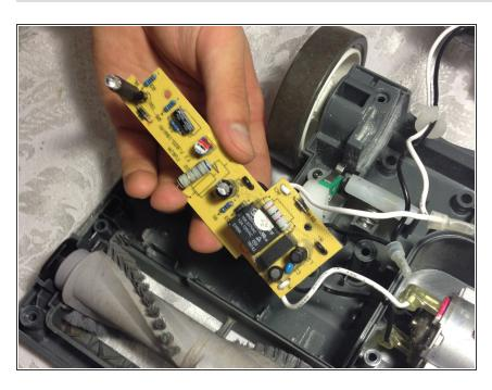
Take out the circuit board and replace with a new one. It may be better to allow a professional to rewire the circuit board to the vacuum.
