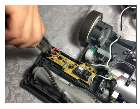
There is one screw at the edge of the circuit board. Unscrew the circuit board before attempting to take it out.
