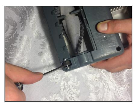
Pop out the two small wheels located on the front end of the bottom of the roller brush compartment.
