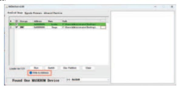
12. Click to execute, and the tool will start flashing the firmware for WiFiLink RX.
