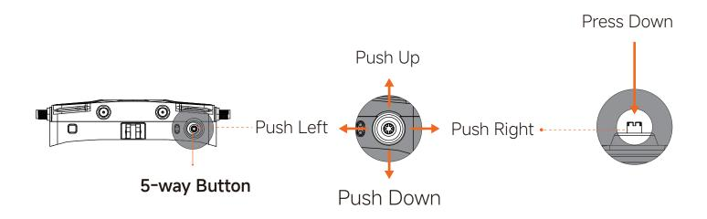
**Ruby System:**Push right to switch OSD interface. Press Down to confirm or open menu. Push up or down to navigate, and Push left to return to the previous menu.
