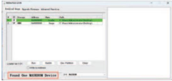
7. When RX enters a flashing mode (MASKROM available), the paths for Loader and Image need to be changed. Click the area shown in the image below to select the "Loader" file.
